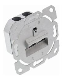
Cat. 6A connection box with 2x RJ45 sockets is surface- or flush-mounted, possessing two LSA connection strips with 8 clamping plates each. Connection box is completely shielded.
